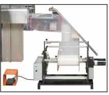
Controlled tension with driven unwind stand to handle large diameter rolls for longer production runs.
